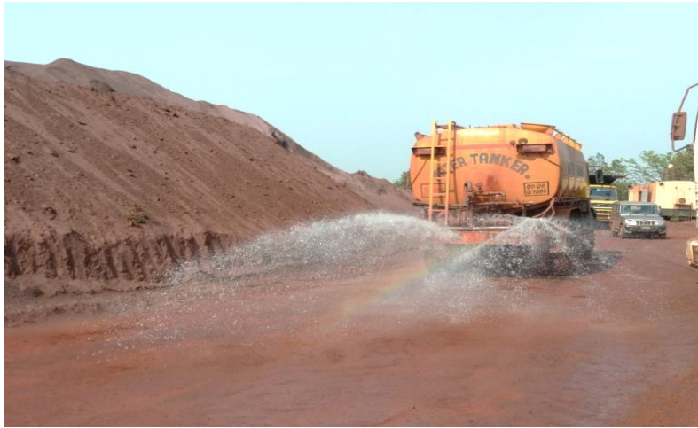
Mobile Water Tanker for dust suppression on mines haul road
